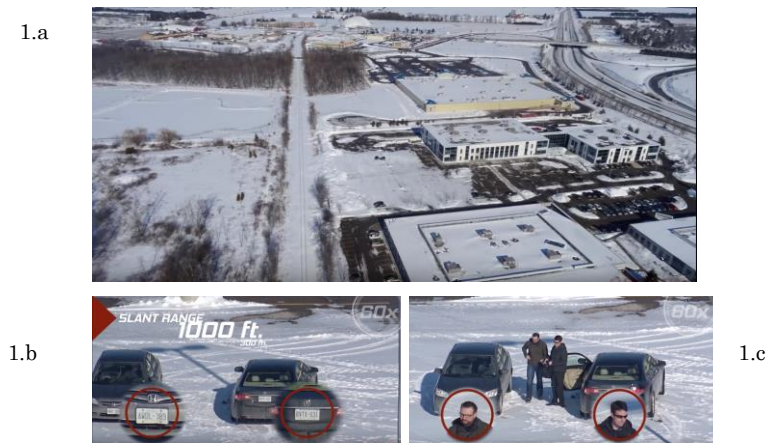
Figure 1: Images from an Aeryon HDZoom30 product demonstration video. Image 1.a. is a still image from a film of a set of cars from a distance of 1000 feet, with the camera not zoomed in. Image 1.b. is the camera zoomed to a magnification capable of reading the license plates on the cars. Image 1.c. is the camera zoomed to a magnification capable of identifying the faces of individuals standing next to the cars. 26
